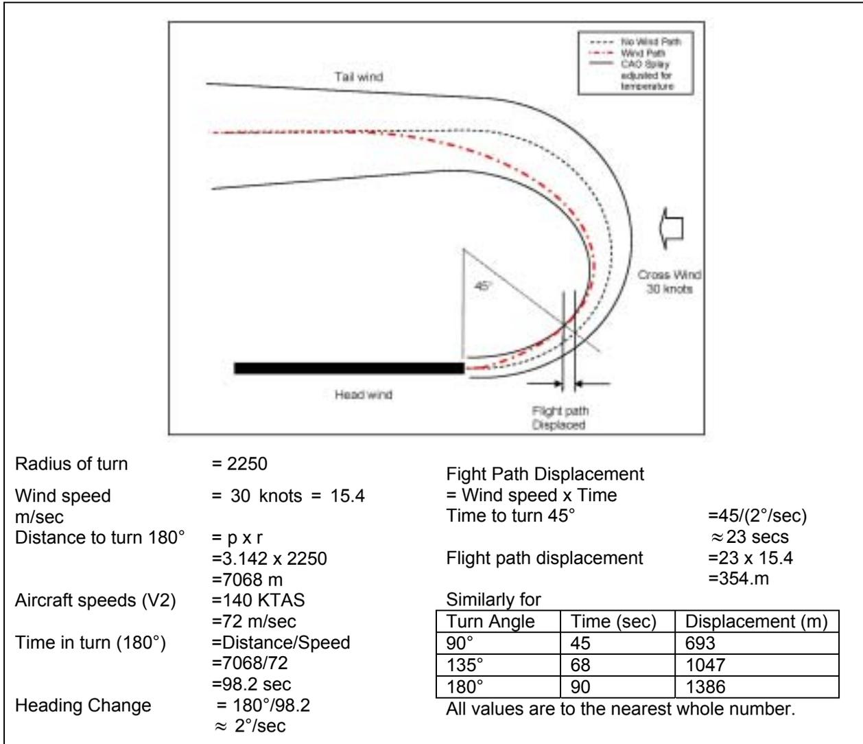
In this example the splay would need to be re-adjusted to account for wind. As previously stated any obstacles that are considered for the takeoff analysis are required to be adjusted to set up an equivalent still air straight out flight path.
