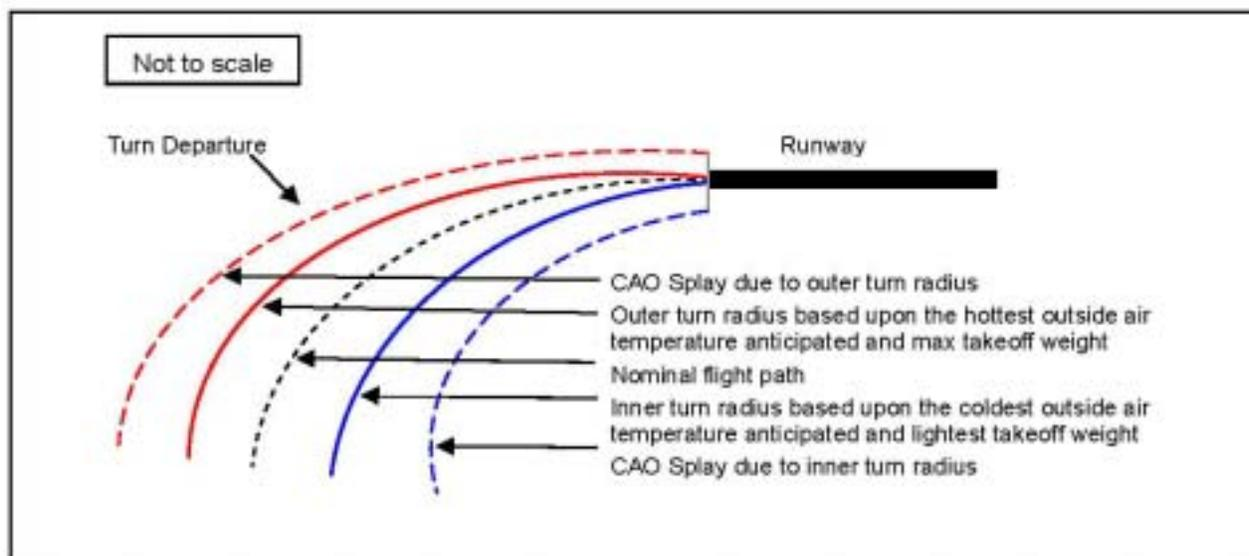
Figure 6.1.1 Splay Design in a Turn
