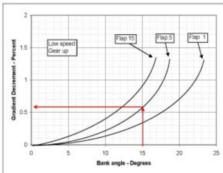
Some EOSIDs require a turn to be performed with a bank angle of more than 15°. In these cases the  $V_2$  speeds may have to be increased (Refer to Improved Climb) to provide an equivalent level of stall margin protection and adequate controllability, i.e.,  $V_{MCA}$  (minimum control speed, air). Prior regulatory approval must be obtained to conduct a EOSID containing a turn with more than a 15° bank angle.
