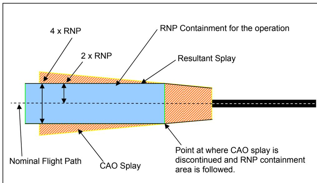
Figure A1.4.1 Path Transition from CAO 20.7.1B Splay to RNP Containment
